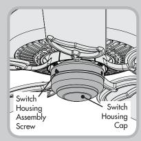
If your fan's switch housing cap resembles this one, remove the whole switch housing by removing the switch housing screws with a Phillips head screwdriver. Remove the two cap screws from the inside of the switch housing. Reinstall the switch housing. Tighten the switch housing screws. Then follow the instructions for TYPE-A ASSEMBLY.
