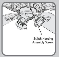
Lift the light kit up to meet the upper switch housing. Install the switch housing assembly screws. Tighten screws.
