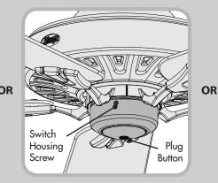
If your fan's switch housing cap resembles this one, remove the whole switch housing by removing the switch housing screws with a Phillips head screwdriver. Remove the plug button. Then follow the TYPE-B ASSEMBLY INSTRUCTIONS.
