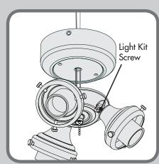
Feed the light kit wires through the center hole in the switch housing. Then attach the switch housing to the light kit by installing the light kit screws into the bottom of the switch housing.
