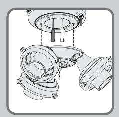
Lift the light kit up to meet the lower switch housing. Guide the two pre-installed light kit screws into the holes in the lower switch housing. Tighten screws.
