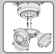
Using the single pin connectors, connect the black or blue wire from the fan to the black wire from the light kit. Connect the white wire from the fan to the white wire from the light kit.
