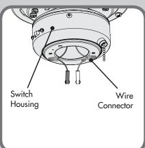
If your fan does not have pin connectors on the wires coming from the switch housing, install the wiring harness provided. Using the provided wire connectors connect the white wire from and connect the black or blue wire from the fan
