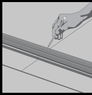
**2** Place the threshold trim under garage door and outline both sides of the trim with a pencil. Trim the length if needed. Ribbed section should make contact with the weather stripping on the bottom of the garage door.
