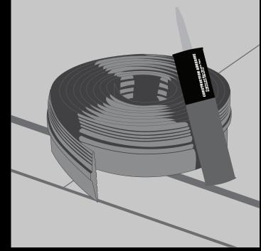
• Threshold kit contains: Threshold trim and tube of adhesive. If the threshold is curled from being rolled, unroll and allow to relax for 2 hours. Allowing it to relax in sunshine may speed up the process.
