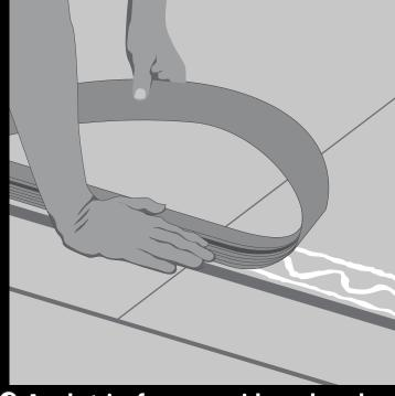
Apply trim from one side and work your way across, pressing trim down firmly as you go. Remove any excess adhesive before lowering the door.
