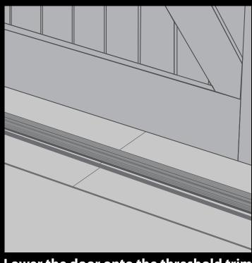
**9** Lower the door onto the threshold trim and allow adhesive to set up overnight.
