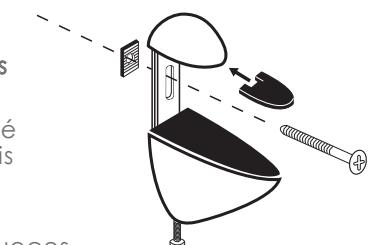
**4** Slide shelf into brackets. Using a screwdriver (for Phillips head screw), tighten set screws to secure shelf.
