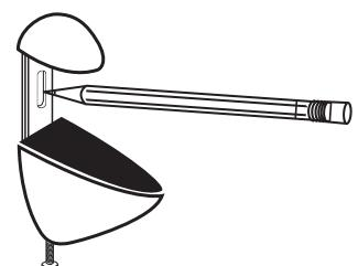
**2** Using a power drill and 9/32" drill bit, drill holes into wall marks. If you are installing into a wall where no studs are available install the drywall anchors after drilling the holes.
