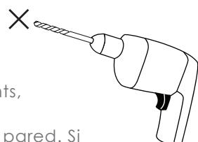
**3** Place each bracket against the wall aligning the bracket hole with the hole on the wall. Using a power drill or screwdriver, (for Phillips head screw), drive provided screws through bracket into studs (or anchors), securing each bracket to wall.
