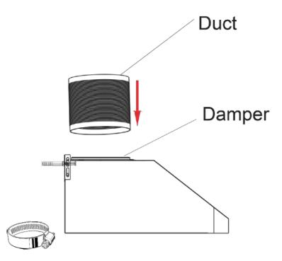
Secure Duct around Damper with Duct Clamp (included)
