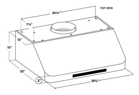
\*actual dimensions may vary slightly by fractional amounts measurements are center to center of each hole
