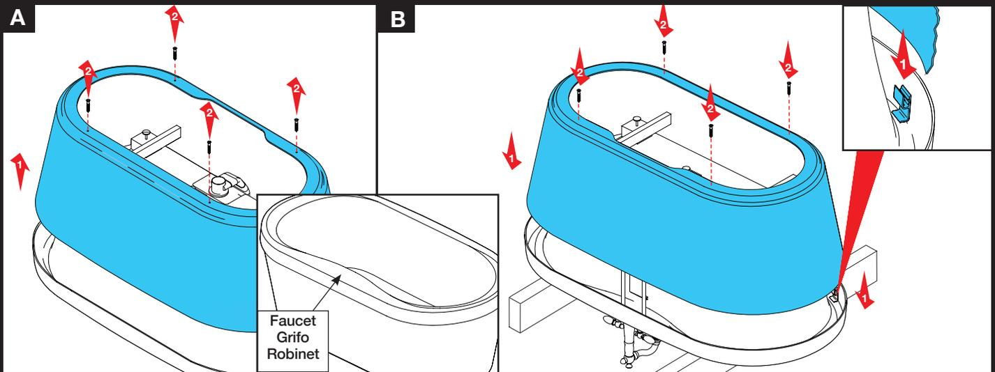
Disassemble the tub prior to installing a faucet. Install the faucet on the bathing well deck.
