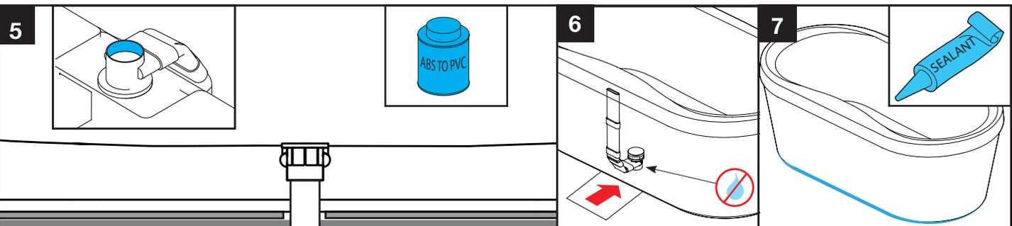
**Please be advised:** This method of joining could violate your local plumbing code. Please refer to your local plumbing code before completing this step. Apply ABS to PVC Adhesive to the inside of the waste drain and outside of the PVC pipe. Set tub back into position making sure to align with the drainpipe. To help with alignment, shine a light down the drain while lowering tub. Apply even pressure while securing position of tub.
