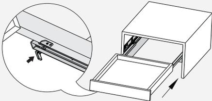
For removal,pull out the locking pin from the drawer side.Lift the drawer and pull it out from the cabinet.
