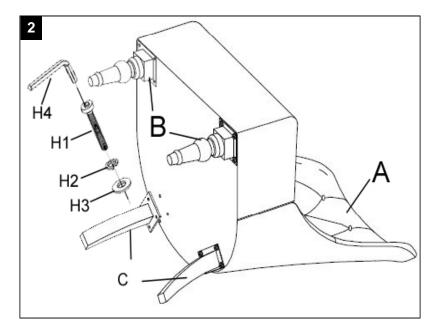
Step 2 Attach rear leg(C) to seat (A), using Allen bolt L(H1), flat washer (H3), and Spring washer (H2),Tighten with allen key (H4)
