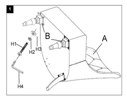
Step 1 Attach front leg(B) to seat (A), using Allen bolt L(H1), flat washer (H3), and Spring washer (H2),Tighten with allen key (H4)
