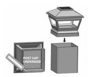
To attach your post cap to the post, apply PVC glue to the underside of the post cap before placing the cap firmly on the post.
