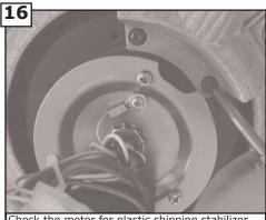
Check the motor for plastic shipping stabilizer tabs, and remove them if they are present. Attach blade assembly to motor using the motor screws and washers provided. Tighten screws securely.
