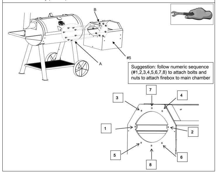
Step 11. Assemble Firebox Bracket (Part #9) using 2 pcs of Bolt M6 x 14 (C) through the holes on Right Front Leg (Part #22) and Right Rear Leg (Part #23). Then use 1 pc of Bolt M8 x 16 (A) and 1 pc of Nut M8 (B) to assemble on Firebox (Part #5)
