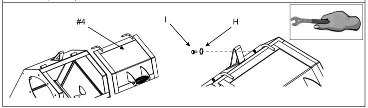
Step 15. Insert Firebox Door (Part #6) onto the Firebox (Part #5). Assemble Firebox Air Vent (Part #8) using 1 pc of Shoulder Bolt M8 x 18 (E), 1 pc of Spring Washer M8 (G) and 1 pc of Nut M8 (B) on Firebox Door (Part #6)
