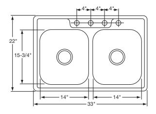
ALL DIMENSIONS IN INCHES, TO CONVERT TO MILLIMETERS MULTIPLY BY 25.4.
