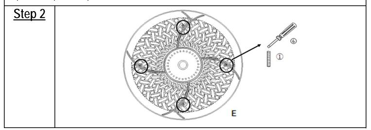
To the underside of the Table Top, there are 4 (four) assembly points. Insert Studs(①) into these 4 (four) positions with Screwdriver(⑥).
