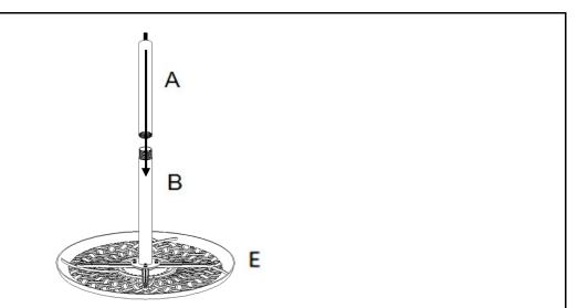
Attach the Pedestal - Lower (A) to the Pedestal(B) by turning the Pedestal (A) clockwise.
