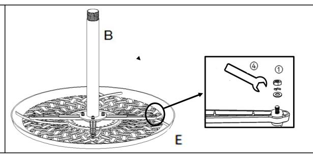
Attach the 'X' Plate, from Step 3, to the Table Top(E).
