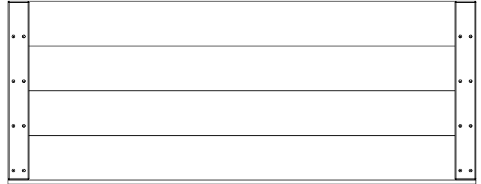
(2) RP1 - ROOF PANEL - W104148
