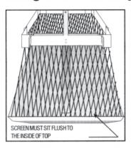
5. With the partially assembled chimney cover still upside/down, place the end screen pieces into position as shown. Make sure they are centered. The screen fits to the OUTSIDE of the braces & bands, snug against the underneath side of top and flush with the outside of the bands.
