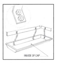
3. Next attach band/brace assembly to inverted top as shown, using 3/8" bolts and nuts. Make certain the marks on bands match marks on inverted top. The bolthead should be to the outside of band (flange side) and top of cover.
