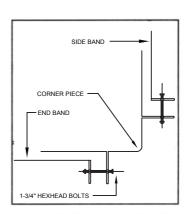
4. Attach the four adjustable corner pieces as shown using sixteen 1<sup>3</sup>/<sub>4</sub>" hexhead bolts and nuts.
