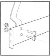
2. Attach the braces to the bands using 3/8" bolts and nuts. After each brace/band unit is assembled place it back in the inverted top until all braces and bands are assembled.
