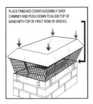
8. Set the fully assembled chimney cover atop chimney. The top of the 2 1/4" band should be level with the top of the first row of bricks on the chimney. There should be a minimum of six inches of space between the top of the flue tile and the inside top of the chimney cover to allow for adequate exhaust.
