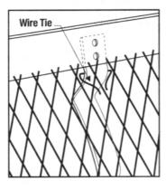
6. With end screen pieces in the correct position, attach the screen at the top and bottom of each brace with supplied wire twist ties by threading the wire behind the brace and back through the screen, then tighten by twisting. Now repeat Step 5 and Step 6 for the side pieces.
