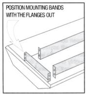
1. Place the four band pieces into the inverted top. Match marks on the bands with the marks on the inverted top. Band flanges MUST be facing out with predrilled holes nearest the inverted top.
