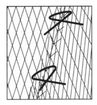
7. To fasten corners together, twist extra tie wires around and through overlapping ends of screens. One or two twist ties per corner is adequate.
