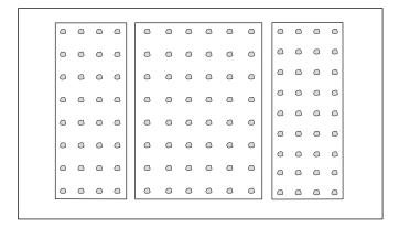
**Note**: When using an industrial grade hot melt glue gun in place of bracing, apply the silicone as stated in Step 2. Then apply the hot melt glue to the panel, as needed, and quickly press the panel firmly into place. Also refer to the **WARNING** on the next page for hot melt glue aplications.
