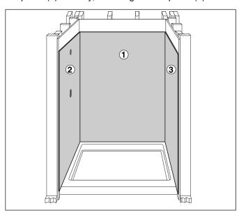
Firmly press the surface of each panel against the wall. It is important to apply hand pressure to the entire surface of the panel to bond it to the wall surface.
