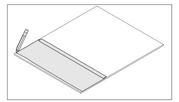
Remove the template and place pieces of masking tape over the area where the saw contacts the Swanstone panel. 4. Cut the panel using a circular saw with a 60-80 tooth carbide blade or a saber saw with a bi-metal blade (14 teeth per inch).
