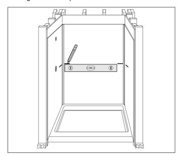
Dry fit the soap dish prior to applying silicone. If the wall is not exactly 90 degrees square, it will be necessary to sand the sides of the soap dish in order to achieve proper fit, using a course grit (60 grit) sandpaper.
