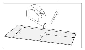
6. Cut clearance holes using a router, saber saw, or hole saw. Drill or cut from the finished side of the panel. For best results, when drilling, place a scrap of wood beneath the hole to ensure a clean cut.
