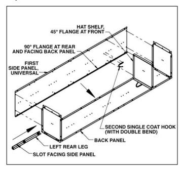
**Step 3:** Attach the second side panel and the right rear leg to the assembly of Step 2. Attach a double bend for the third single coat hook and install the coat rod as shown on page 3. The locker chassis is now complete.
