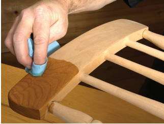
Apply wax in small sections
