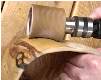
Use brush sleeve to spread wax
