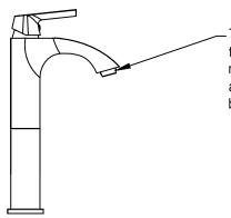
Twist open the aerator cover counterclockwise to remove the aerator. You will find an aerator installed here. Simply remove the 1.2 gpm aerator and replace it with the 1.5 gpm aerator (provided). Replace the aerator cover by twisting it back on clockwise.
