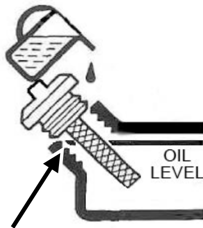
Figure 2 - Add Oil To TOP Of Threads
