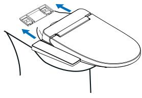
Secure the remote control holder to the wall with screws or peel off the double-sided tape sticker on the back of the remote
