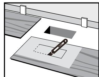
**Note:** Be sure to leave a minimum of  $\frac{1}{4}$ " (6mm) expansion space around all fixed objects, cabinetry, and metal door jambs.
