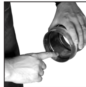
Figure 5: Check for EPDM seal
