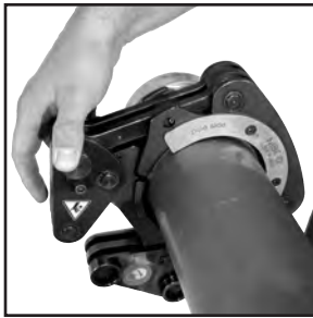
Figure 6: Placement of the pressing chain onto fitting or valve
