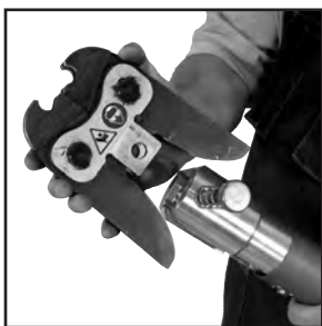
Figure 7: Placement of adapter jaw into the tool
