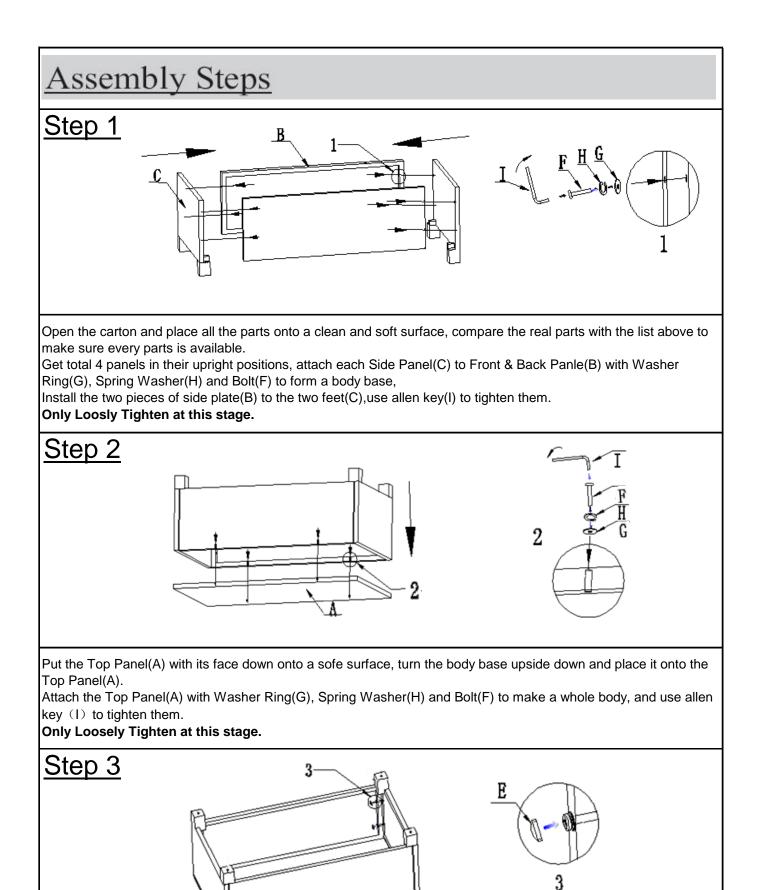
Tighten all Bolts completely, put the Plastic Cap(E)to cover the Bolt heads.
