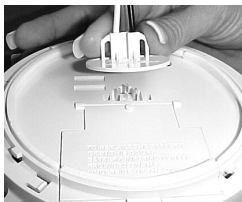
FIGURE 4 Installing AC Quick Connect
