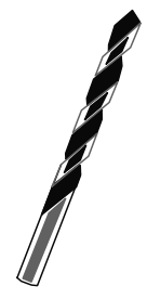
9/16" Drill Bit Longer than Diameter or Thickness of Post
