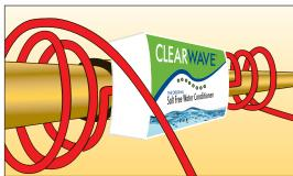
Coil one red antennae counter-clockwise, the other clockwise, and fasten with supplied tiewraps or electrical tape. The tighter the antenna are coiled, the better ClearWave functions.
