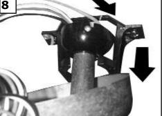
Hang assembled fan from the mounting bracket installed to ceiling in previous steps. Mak e sure the fan is hanging straight. Rotate fan until the tab on the Mounting bracket engages the slot on the Downrod Ball. This must be done to prev ent the fan body from rotating when the blades are in motion.
