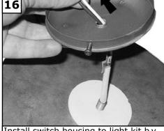
Install switch housing to light kit by turning clockwise to tighten.
