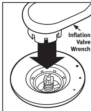
**If the valve is difficult to turn, remove the valve completely and add a small amount of silicon grease to the valve O-ring and reassemble.**
