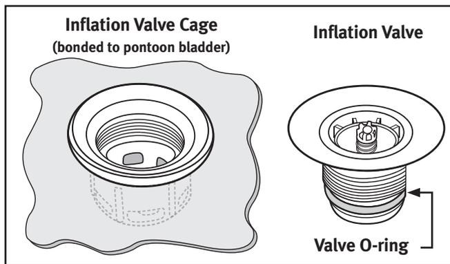
The inflation valve consists of a two-part assembly. There is the inflation valve itself and the inflation valve cage. The inflation valve cage protects the inflation valve from damage and is bonded into the pontoon bladder.
