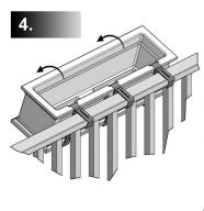
Hang the window box on the railing. Push the bracket extension tight against the hand rail and tighten the bolts with a wrench. Make sure all fasteners are firmly tightened.
