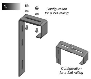
Assemble the bracket and extension piece using the carriage bolts, 1/4 inch washers, and acorn nuts as shown above. Adjust the width of the extension to match the railing. Hand tighten to hold the bracket in place. For larger railings over 5 inches wide only 1 bolt can be used to attach the bracket extension.
