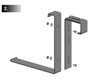
Align the deck rail bracket with the wall mount brackets that shipped with your Mayne window box. For the Yorkshire window box align the bottom 2 slots on the deck rail bracket with the Yorkshire wall mount bracket. Fasten them together using the #12 Hex Bolt, #12 Washer, and #12 nut. Tighten firmly with a wrench.
