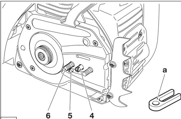
Remove the plastic transport cover (a) and dispose of properly.
