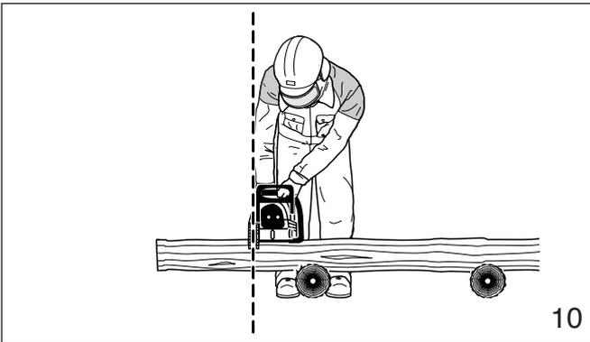
Position the chain saw in such a way that your body is clear of the cutting attachment whenever the engine is running (fig. 10).
