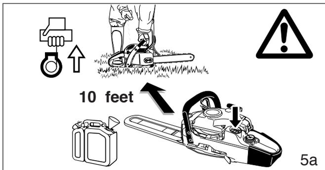
Wipe off any spilled fuel before starting your saw and check for leakage.
