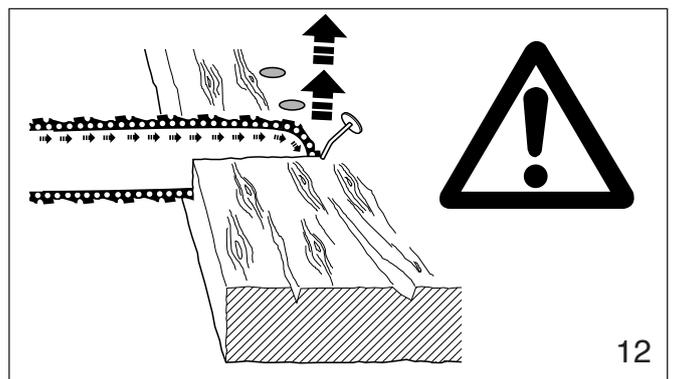
This reaction can occur in a fraction of a second and under some circumstances, cause the guide bar and chain to strike the operator with enough force to cause severe or fatal injury. It may also occur during limbing. It also occurs when the nose of the guide bar is pinched unexpectedly, unintentionally contacts solid material in the wood (fig.12) or is incorrectly used to begin a plunge or boring cut.
