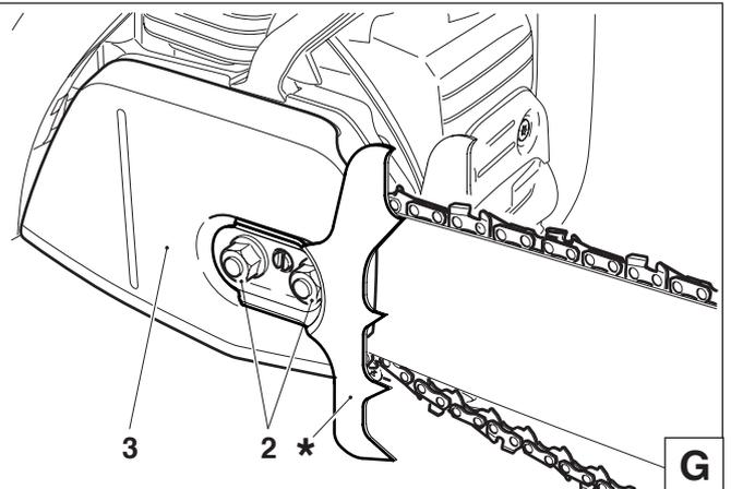
**Tightening the saw chain**
