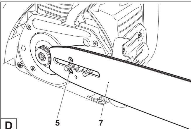
Put on the guide bar (7). Make sure that the pin (5) of the chain tensioner engages in the hole in the guide bar.
