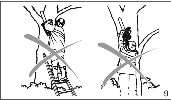
In order to keep control of your saw, always maintain a firm foothold. Never work on a ladder, in a tree or on any other insecure support. Never use the saw above shoulder height (fig. 9).
