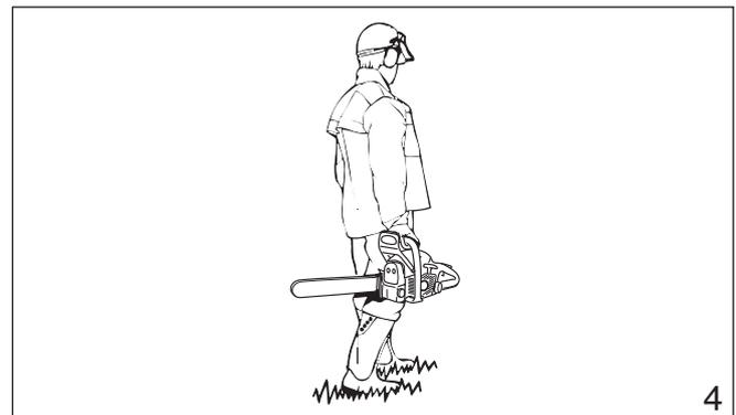
**By hand:** When carrying your saw by hand, the engine must be stopped and the saw must be in the proper position.
