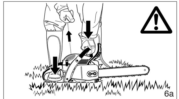
Place the chain saw on firm ground or other solid surface in an open area. Maintain a good balance and secure footing. Place your right foot through the rear handle opening and firmly grasp the front handle with your left hand (fig. 6a).
