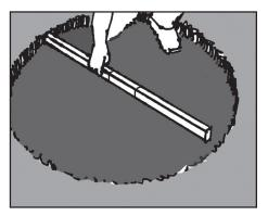
2. Check the level of the soil inside the circle in all directions. Remove soil from the high spots to bring it close to level.
