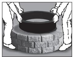
8. Next, lower the fire pit liner inside the blocks. The outside flange of the ring should be centered and rest on the inside edge of wall block units.
