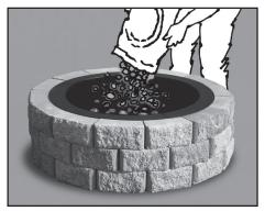
**9.** After the adhesive cure time has lapsed, pour lava rock into the fire pit until the level reaches the bottom of the fire ring liner.
