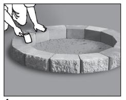
**4.** Place 14 wall block units on top of paver base. Lay them tightly together to form the circle. Level each stone front-toback and side-to-side. Make sure each stone is even with the previously leveled block. Use a rubber mallet to level.
