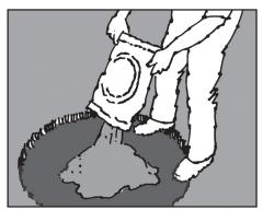
3. Add 1.5-2 inches of paver base to your circle and rake it level. Using a tamper, pack the entire area of paver base until firm. Make sure the surface is level before laying blocks.
