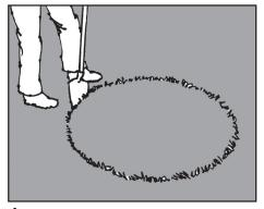
**1.** If putting your fire pit on a lawn, mark a 40-inch diameter circle and remove all sod and roots inside the circle. Dig approximately 2 inches deep. If putting your fire pit on a patio, mark the circle with chalk and skip ahead to step 4.
