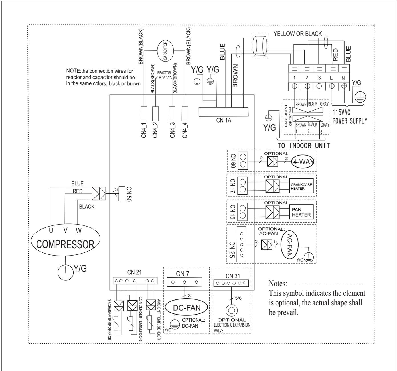
Figure 41 Outdoor unit wiring diagram example (refer to unit for actual wiring schematic)
