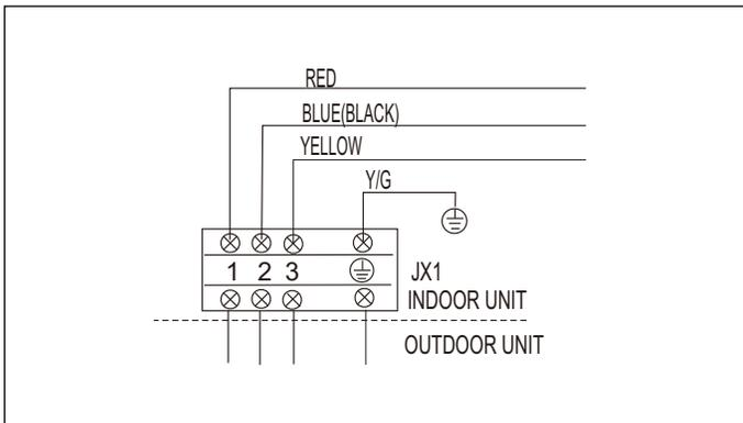
Figure 18 Wiring Schematic example (refer to unit for actual wiring schematic)
