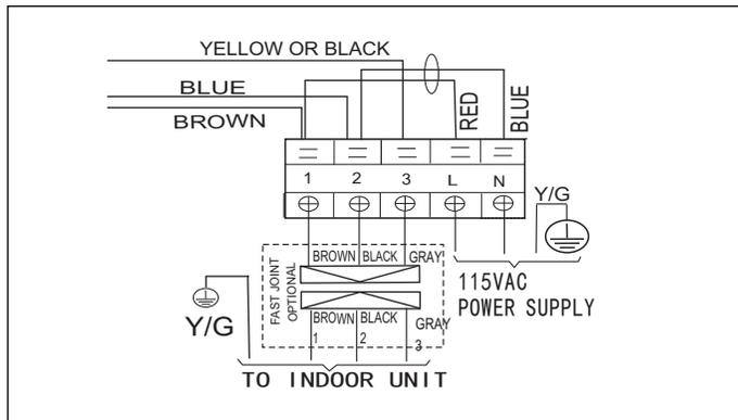
Figure 25 Wiring schematic example (refer to unit for actual wiring schematic)
