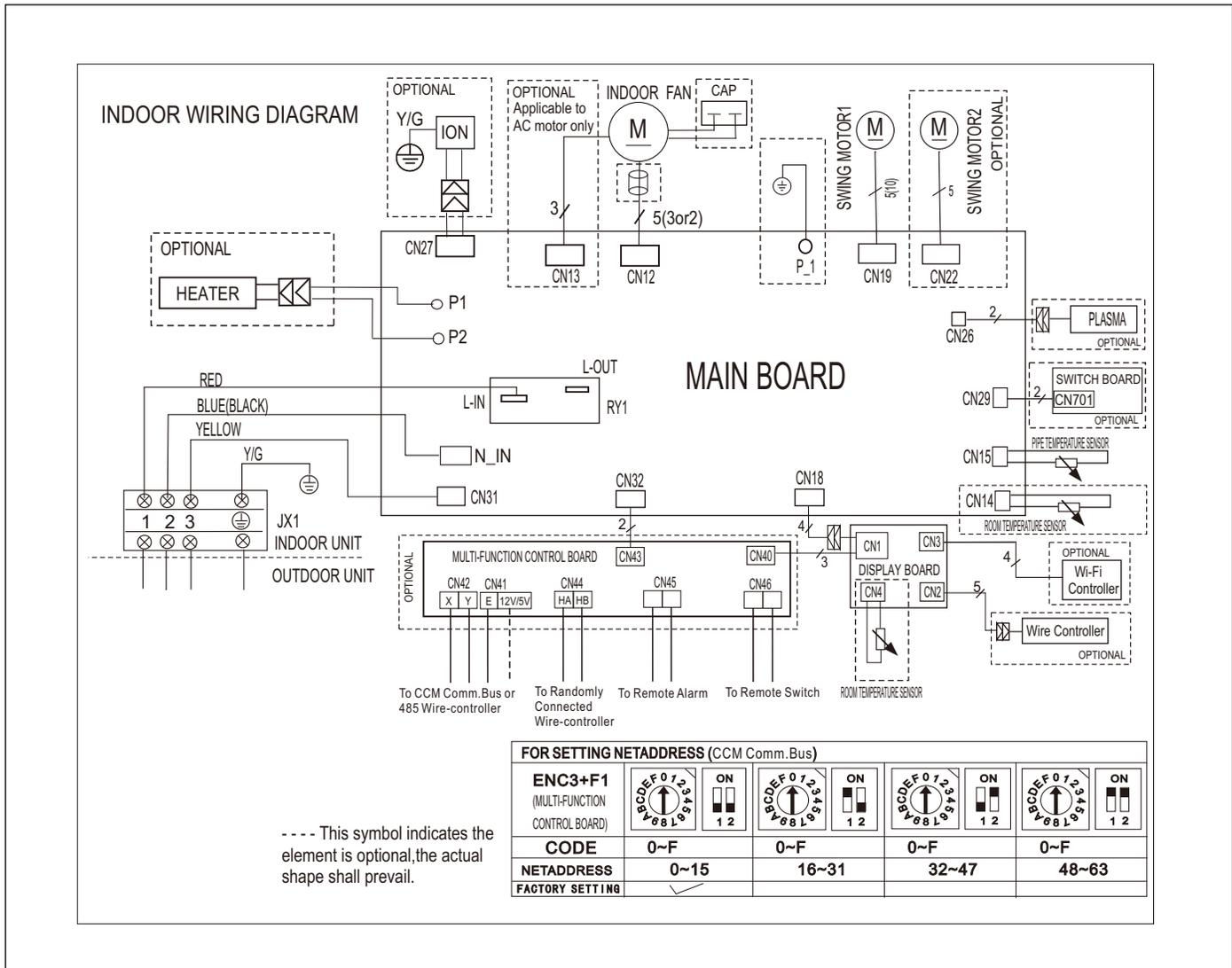
Figure 40 Indoor unit wiring diagram example (refer to unit for actual wiring schematic)
