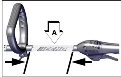
1. Position Support Handle (A) in comfortable operating position and tighten wing nut (B). The cutting attachment should be 5 - 7.5 cm (2 - 3 in.) above the ground and as level as possible.
