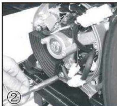
② Remove the 2 bolts holding the AVR.
