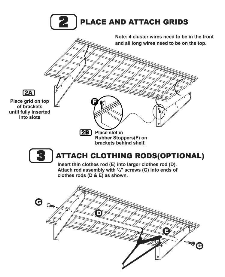
You have now completed the installation are ready to load your new HyLoft Shelf. (Maximum 150 lbs. per 18" x 36" unit, evenly distributed). Place the sticker provided on a bracket for easy access to reference information.
