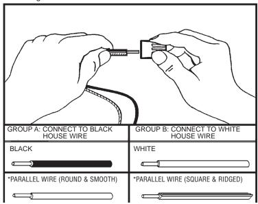
\*NOTE: When parallel wire is used, the tracer wire is square shaped or ridged, and the less tracer wire is round in shape or smooth. (Seen best when viewed from wire end.) To separate wires, grasp the ends of each wire and pull apart.
