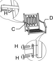
Connect armrests (C) and (D) with chair back (A) and seat board (B). M6\*20 bolts (H) are used.
