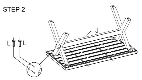
Screw table leg support (J) to table legs (I). M6\*50 bolts (L) are used. Please do not tighten any screws at first. Make sure all screws are inserted properly. Tighten all screws to the end.
