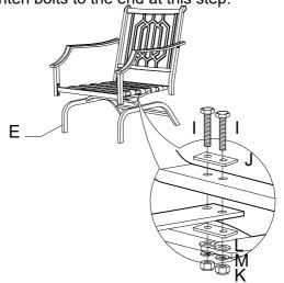
Connect chair base (E) with assembled seat part. M8\*40 bolts (I), spring washers (M), washers (L) and nut (K) are used. Please make sure all bolts are inserted and connected properly, then tighten all bolts to the end.
