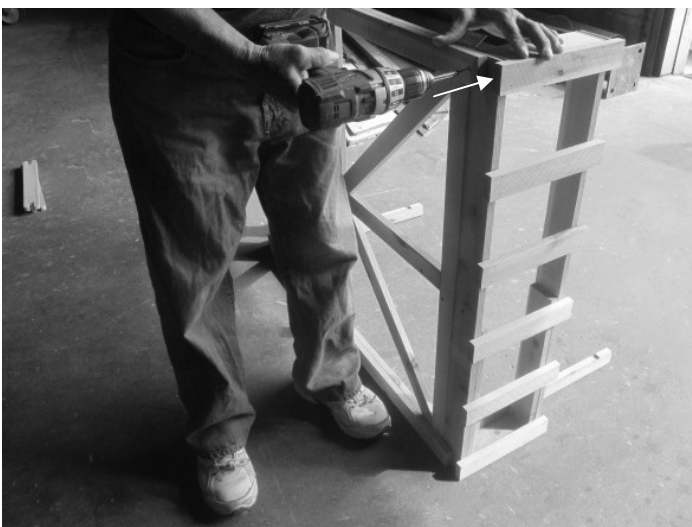
5. Place the back frame on the back of the bottom arbors. Match numbers for the best result.
