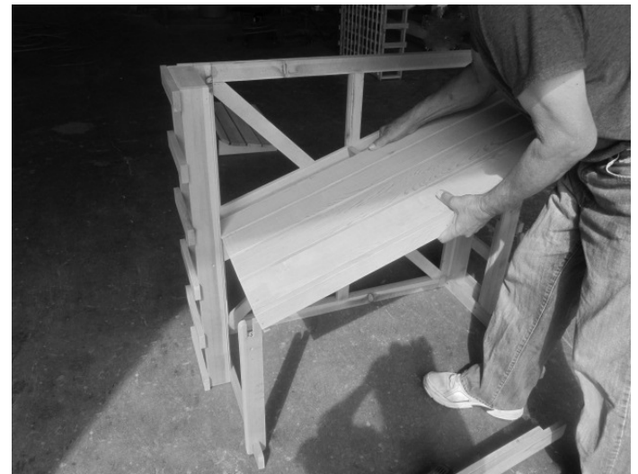
10. Install the bottom bench between the bottom arbors. Match numbers for the best result.
