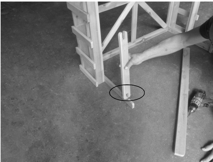
9. Find two vertical bench legs with matching numbers. Fasten the both bench legs with screws.
