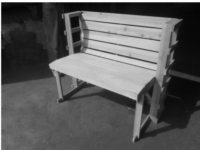
11. Place the top bench between the bottom arbors. Match numbers for the best result.
