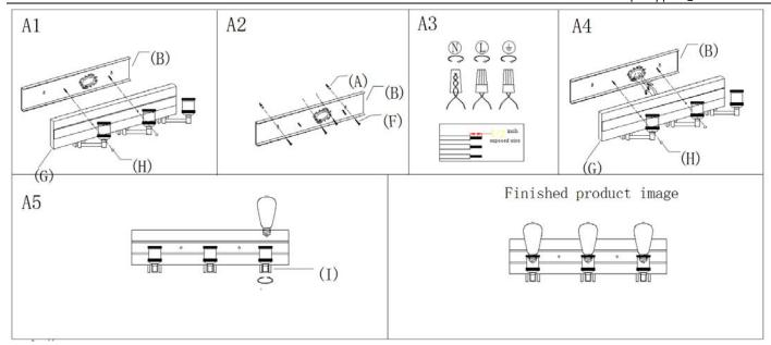
Step A1: Unscrew the knob nut(H) from back plate(G) then gently remove mounting plate (B)
