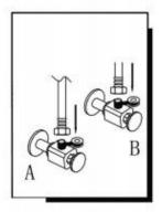
3.Attach two flexible hoses to water supply.
