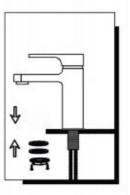
Install faucet through center hole, assembly washer and metal washer onto faucet, and tighten with lock nut.
