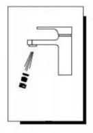
4.After installing faucet, remove aerator assembly and open the hot and cold water supplies. Check for leaks.Turn on faucet handle for one minute to flush debris from faucet.Close the handle and re-assemble the aerator.
