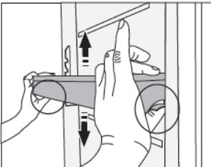
The height of the door bins/shelves can be adjusted to your preferences without having to take them out of the appliance. Gently squeeze the tabs on both sides and move the bin/shelf up or down. To remove a bin from the appliance, lift it as far as it will go and pull it out.
