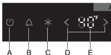
Use this function if you do not wish to manually adjust the appliance settings. To activate, press and hold the **B** key (for three seconds); **LL** will appear on the display **E**. This will lock all keys except **B**. To deactivate the safety lock, press the **B** key and hold it for three seconds.
