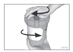
Align VacuValve on cup cover with Prime Pump/Spray knob. Push cup assembly onto sprayer and twist to lock.
