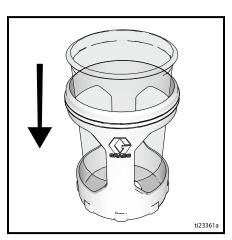
Fill FlexLiner with material. Securely tighten cup cover onto cup support. For proper sprayer operation lid must seal tightly with the cup.
