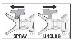
While holding the sprayer upside down point the sprayer into a waste pail. Pull the trigger for three seconds.
