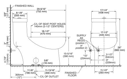
IMPORTANT: Water supply on the wall is required at 2-1/2" (64mm) or 9" (229mm) from centerline of the toilet (see rough-in). First suggested position is hidden behind the toilet. The geometry of the toilet gives space for this installation. The second suggested position is next to the toilet. Between these two positions, the space for the supply between wall and toilet is limited to 4-7/8" (124mm). In this case, check your supply and hose dimensions.
