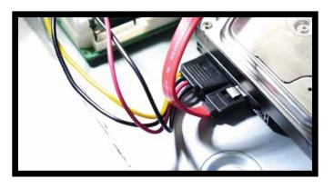
Attach the DVR/NVR casing using the screws removed in **STEP 1**. Some DVR/NVR models will have a plug that must be reconnected to the unit.
