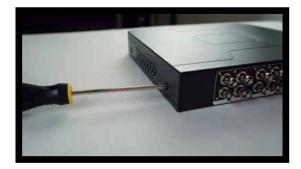
Carefully hold and lift the casing from the back panel. Lift upward and toward the front panel of the device.
