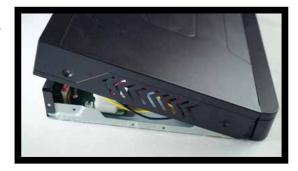
Disconnect the Data Cable and the Power Cable from the HDD. This **MUST** be done slowly to avoid any internal damage to the System.
