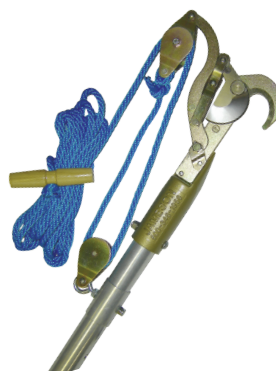
JA-14 DP Double Pulley Pruner Double pulley allows for additional leverage and significantly reduces pulling force required (Adapter Included)
