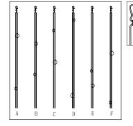
The strands are attached to the fixture in the sequence of A, B, C, D, E, and F. If a strand becomes unattached, it can be clipped back on.
