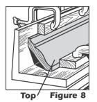
As described, crowns do not lie flush against the wall. Cutting correct 45° mitres is critical. Clamp two blocks of wood to the mitre box to hold the moulding in place at the angle at which it will be installed. Once blocks are in place, insert moulding prior to cutting, face out and upside down (Fig.8). Then cut
