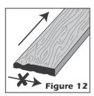
Use a fine grit sanding sponge or at least a 220-grit sandpaper on a sanding block. Always sand with the grain of the wood (Fig. 12). Coarser grits of sandpaper, or going across or against the grain will tend to leave fine gouges that may be visible through subsequent
