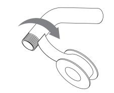
Thread Showerhead onto shower arm by turning it in a clockwise direction. Tighten with adjustable wrench. Turn water supply on and check for leaks.
