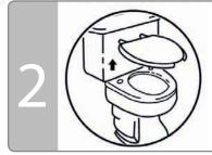
Remove existing seat and lid. Release the bolts on both sides of the existing toilet seat.
