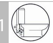
Shut water supply off by turning it to the right and disassemble the water hose.
