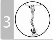
Connect supplied universal 7/8" T valve to the fill valve underneath of toilet water tank and connect water supply hose between universal 7/8" and shut off valve
