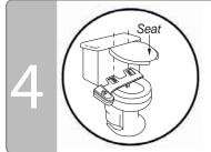
Mount bidet and toilet seat/lid over toilet mounting holes. Supplied rubber O-rings should be placed under the bidet mounting bracket to protect and secure the bidet on the toilet.
