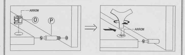
NOTE: • THE ARROWS ON THE HIDDEN CAM-LOCKS SHOULD POINT TO THE CAM-BOLTS
